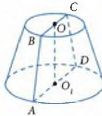
$$V = \frac{1}{3} \pi H (R_1^2 + R_1 R_2 + R_2^2) = \frac{1}{3} \pi \cdot OO_1 (BO^2 + BO \cdot AO_1 + AO_1^2)$$
