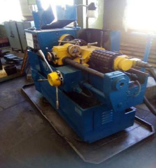
A smaller industrial machine with a blue and yellow frame, featuring a revolver turret and a lathe bed, situated in a factory setting. | Токарно-револьверный 1Д325             | Договорная      |
