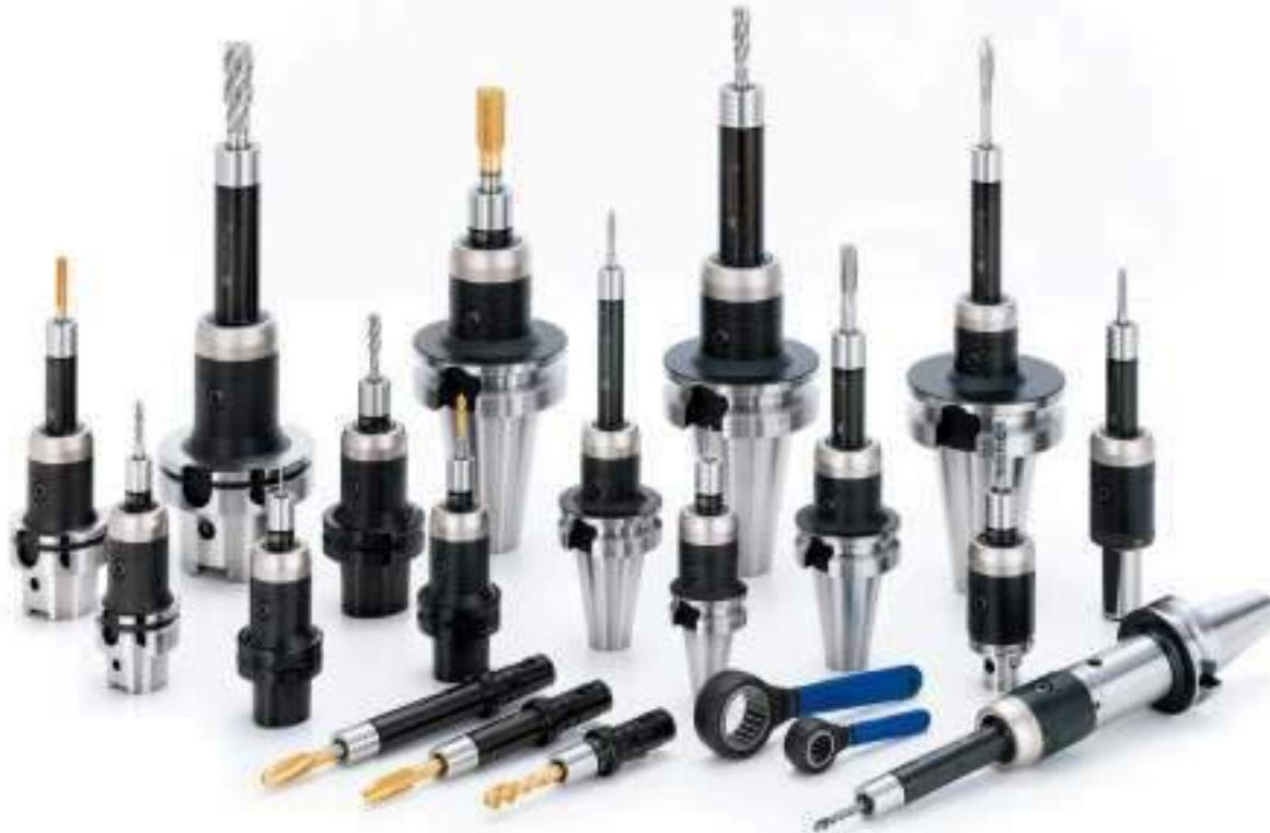
**BIG MEGA SYNCHRO Tapping Holder compensates for synchronization errors with any type of tap. Minimized thrust load to both the tap and workpiece improves thread quality and tap life.**
