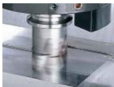
Finishing surface roughness was Rz=2.53 at V=200, F=0.15 cutting data.
