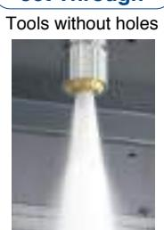
Unique sealed collet nut for coolant-through tools.
