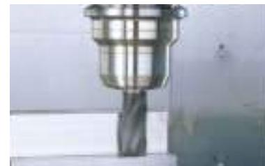
Flange contacting nut and simultaneous taper & flange contact assure highest rigidity.
