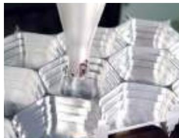
For less rigid workpiece with 3mm thickness clamped by a vise, feed rate of 4,300mm/min on both sides of the workpiece is achieved.
