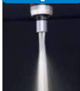
Coolant is supplied through both the tool and the slits of Tap Holder.
