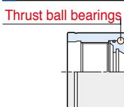
Thrust ball bearings to eliminate distortion of the collet during tightening. Patented design prevents ball bearings from moving at high speed. Threads are finished after heat treatment.
