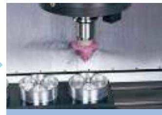
Wind pressure cleans workpieces.
