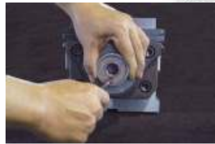
Now to adjust the clamping force
