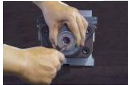
Now to adjust the clamping force
