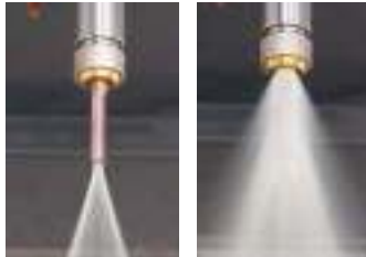
With PS RING Without PS RING
