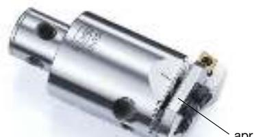
粗搪孔刀本體、粗搪孔刀座 Body and Cutting Insert Holder
