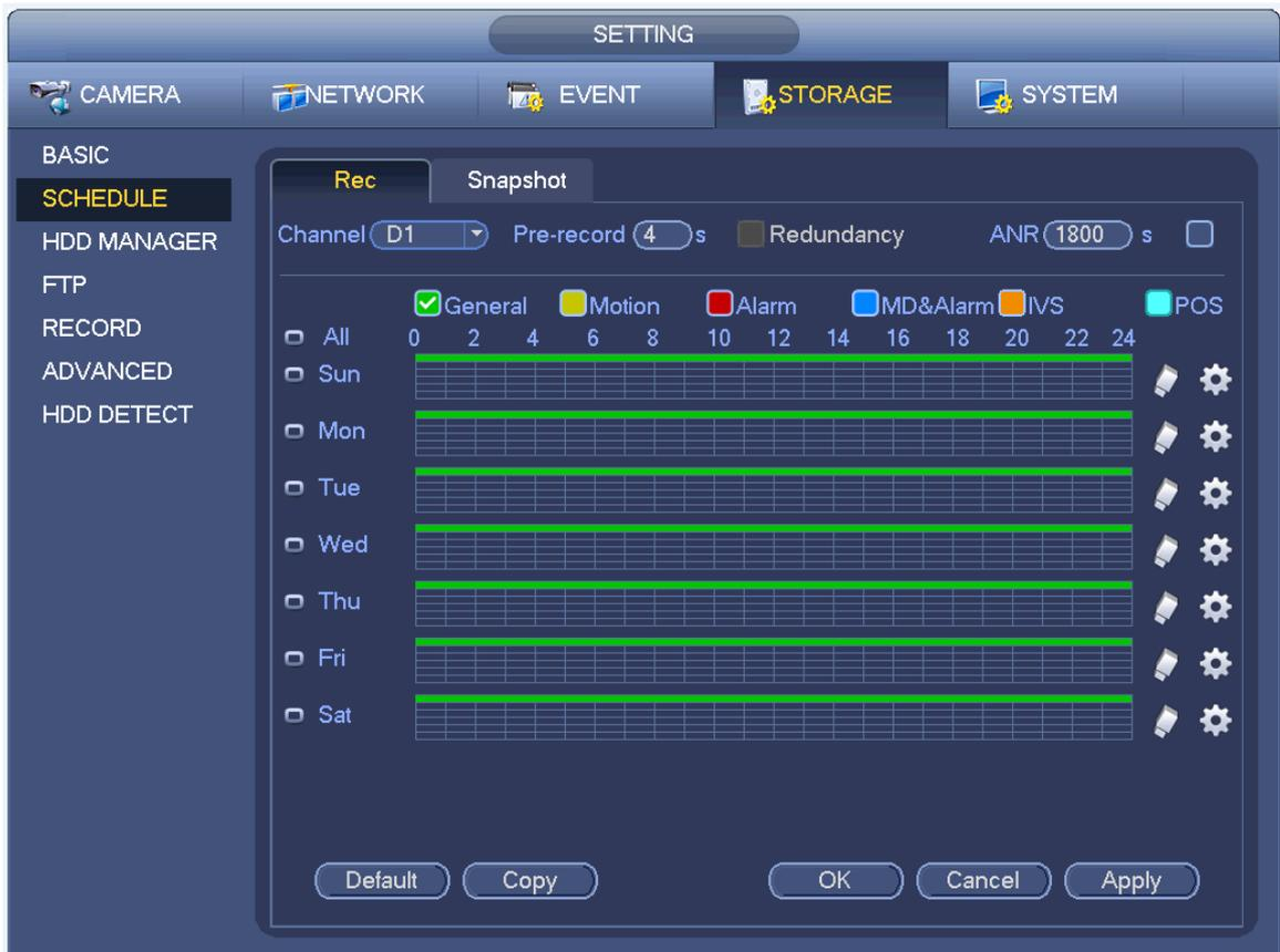
**Step 2** Configure parameters such as channel, pre-record, ANR and record type.
