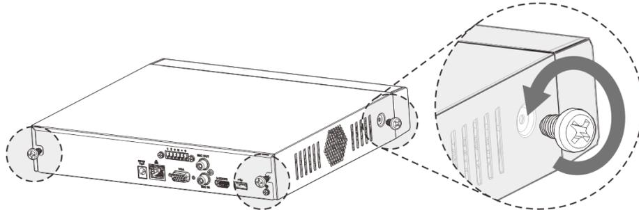
**Step 2** Remove the case cover along the direction shown in the following arrow.
