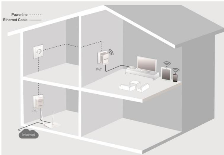
AV1000 AC Wi-Fi Powerline Extender Kit extends 650 Mbps dual band WiFi to any room in your house using existing electrical wiring. With 1000 Mbps Homeplug AV2 powerline technology and gigabit Ethernet port, PH10 can offer better HD/UHD IPTV and online gaming experiences.
