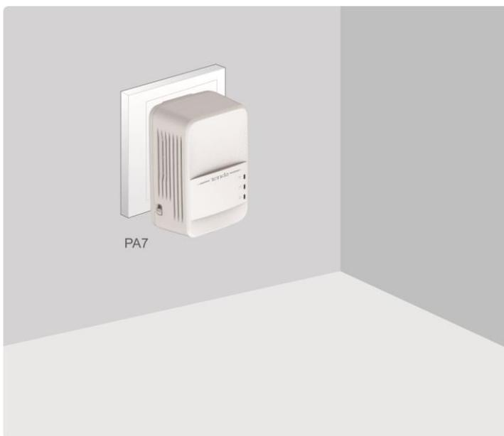
**Step 2** Connect PA7 to your wired device, such as a set-top box of a TV, and plug it to a wall receptacle nearby.
