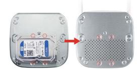
2) Fix the HDD on the bottom pannel with screws.
