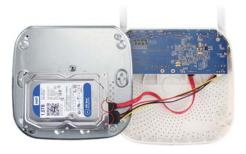
3) Connect data wire and HDD wire between PCB board and HDD.
