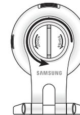
2. Remove the bracket from the main body of the camera, as shown in the figure below.
