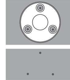
3. On the mark, drill a hole to a depth of about 3cm in the wall using a drill bit and drill with a 5mm diameter for concrete. Remove any debris remaining in the hole after drilling.
