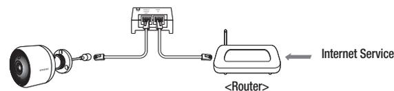
3. When the camera is connected to the router, the LED turns blue. (Connection standby time: 30 seconds maximum) If the LED does not turn blue, return to Step 2 and confirm that all steps were performed correctly.
