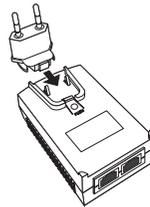
2. To remove the power plug from the PoE adapter, press the [PUSH] section as shown in the figure below, and push up the power plug.
