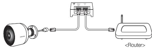
4. Connect the LAN cable from the PoE adapter [DATA IN] socket to the LAN port of the router.
