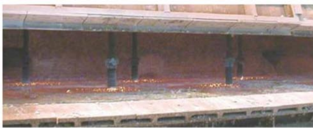
Figure 4. 6 rotor IRMA assembly in a 70 T furnace. Note: in normal operation, the door is closed.
