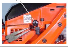
1. Take off plug (C) for adjusting L and H mixture needle. Turn the L and H mixture needles out anticlockwise to rich stop, and meet limiter caps tabs (A) with locating slots (B).
