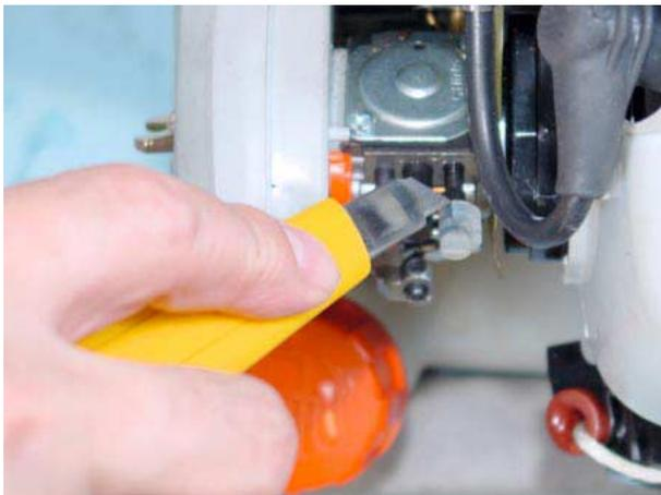
1. Turn L mixture needle clockwise until lean stop to cut easily.
