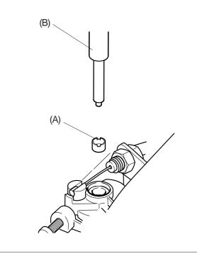
6. After adjusting carburettor, insert and secure plug (A) deep in the needle hole per the directive. 2 way limiter cap tool (B) is useful to insert the plug.
