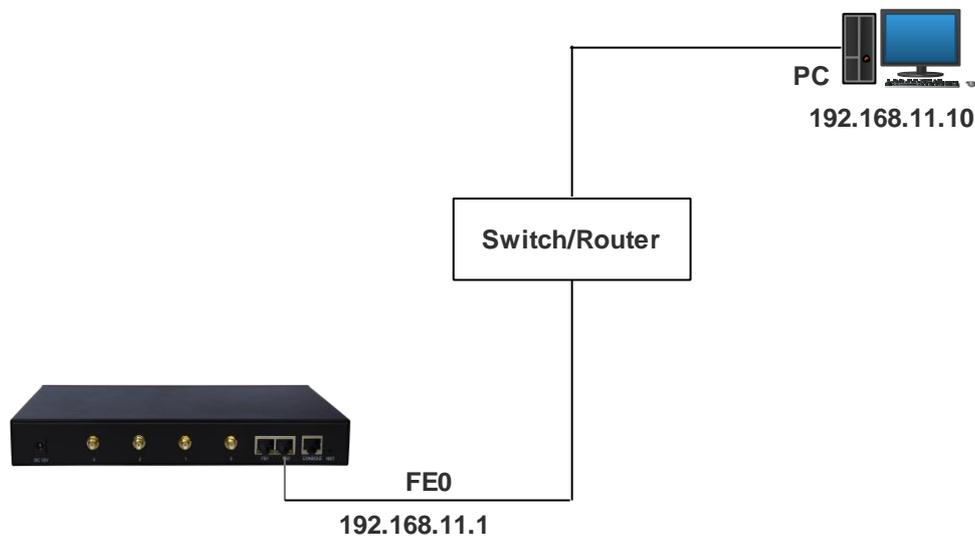
**Note:** DWG2000EFG has two Ethernet ports (namely FE0 and FE1). The device can work normally when either of the ports is connected to PC. The IP address of DWG2000EFG must be at the same network segment with that of PC.
