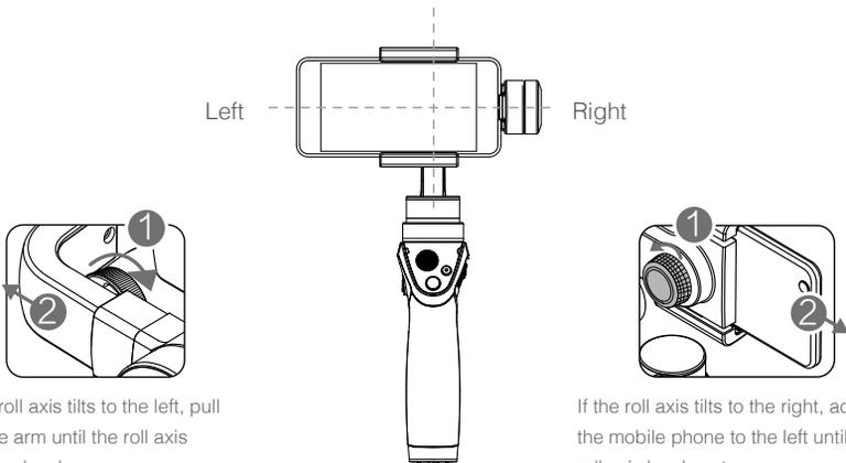
If the roll axis tilts to the left, pull out the arm until the roll axis remains level.
