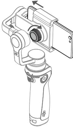
2. The system is balanced if the mobile phone remains level when released, balanced only by the gimbal.
