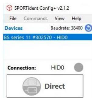
After connecting a BS11 station with the USB cable to the computer, it can be configured with Config+. The station is read by double clicking on the device in the start-up screen (Direct and Remote are not active).
