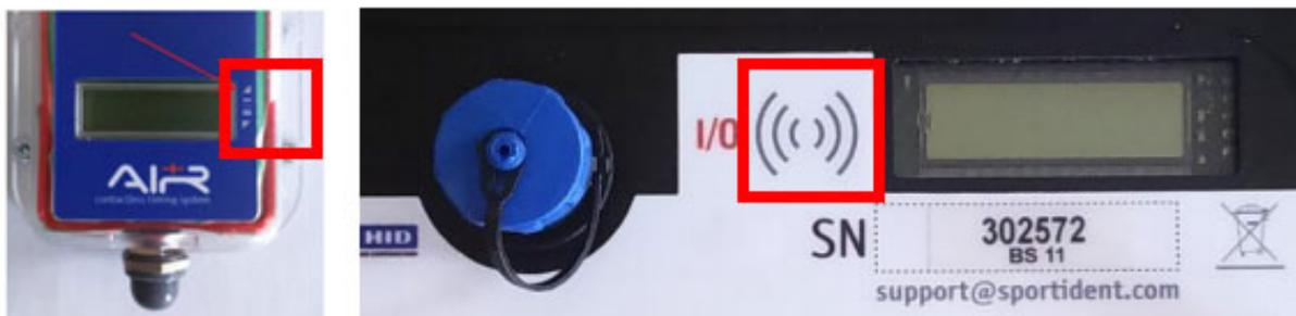
The stations initialise with an acoustic and optical signal. The display is active. Additionally, there are repeating short optical feedback signals while the station is active.
