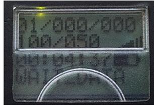
When switching the SIGSM-DN on, information becomes available on the LCD display. A green LED is blinking, confirming that the GSM is on.
