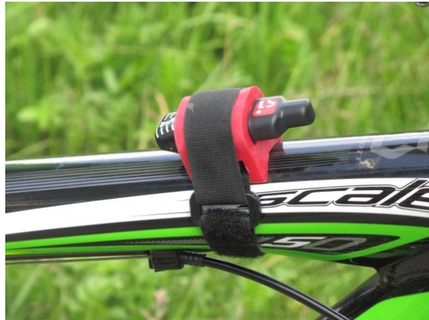
For MTB applications we recommend carrying the SIAC on the wrist or using the **SPORTident Mounting holder "Bike"** to affix the card on the frame or handlebar of the athlete's bike. Please ensure that the SIAC is mounted at the height of the field stations used for the event.
