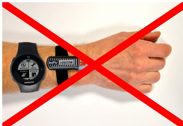
The AIR+ mode can be compromised by disturbances caused by third party equipment. The active antenna of some GPS watches can significantly reduce the SIAC's sensitivity. As a rule, a GPS watch and SIAC shall not be carried on the same arm.
