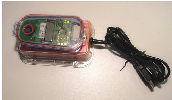
Put the coupling stick (ferrite for faster transmission) into the USB station and place the station (in service mode) on top of it (this station becomes the slave station).
