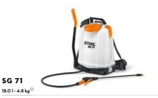
Backpack sprayer for professional users. Increased user comfort with option to mount pump lever on either side, as well as width and length adjustment. High-quality straps and moulded back panel make it very comfortable to wear. Ergonomic shut-off valve with pressure gauge. Approx. height 55 cm, approx. width 50 cm, approx. depth 22 cm.
