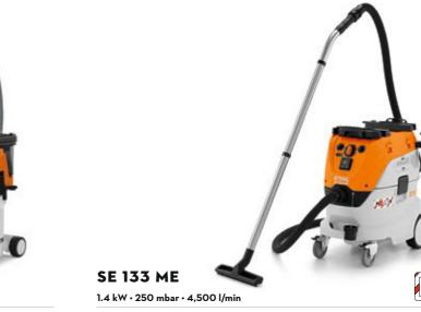
Powerful wet/dry vacuum with automatic switch-on function in dust class M. Automatic filter cleaning without loss of suction power, automatic volume flow monitoring, infinitely variable speed control, with adapter plates for carrying tool boxes, anti-static accessories also for extraction on battery-powered/electric power tools.
