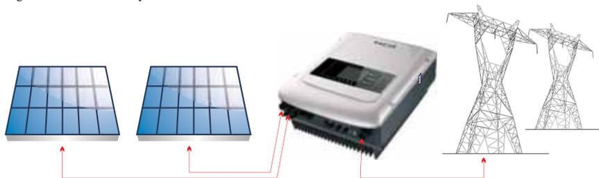
Sunny Deer series inverters can only be used with photovoltaic modules that do not require one of the poles to be grounded. The operating current during normal operation must not exceed the limits specified in the technical specifications. Only the photovoltaic modules can be connected to the input of the inverter (do not connect batteries or other sources of power supply).
