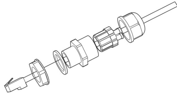
**Step 4** Crystal plug with RJ45 crimping tool.
