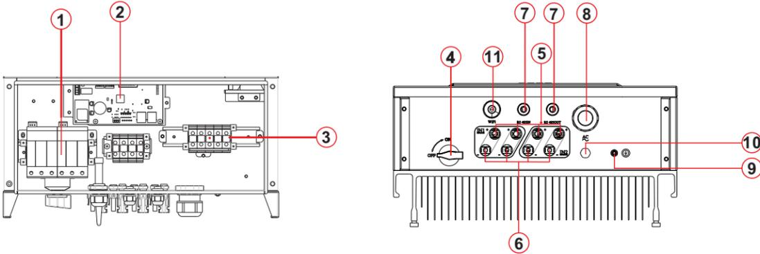
1. DC SPD 2. Communication card 3. AC output terminal 4. DC switch
