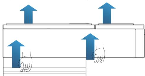
**Step 2** Lift the Sunny Horse Series from the packing case and move it to the installation position.
