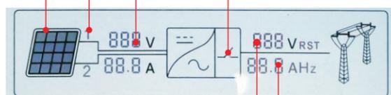
A16 - Indicates R/T/S phase current or frequency and displays in turns in every three seconds
