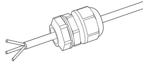
**Step 3** The cable stripped to the corresponding stem node hole.
