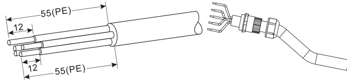
**Step 3** Connecting the AC output power cable: The AC output cable (R,S,T,N and PE) is connected to the terminal block, as shown in figure 4-7.
