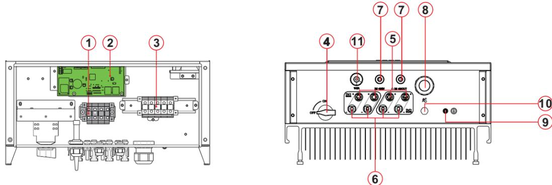
1. DC input terminal 2. Communication card 3. AC output terminal 4. DC switch 5. DC positive poles connectors
