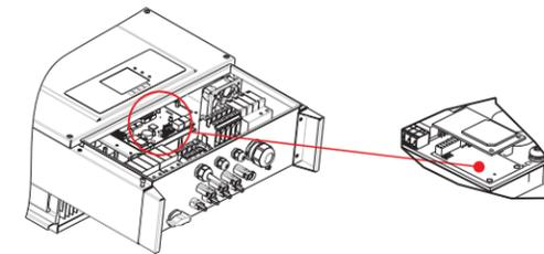
**Step 3** Screw out the sealing nut corresponding, to let the antenna expose a portion, and tighten the screw nut.
