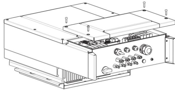
**Step 2** Remove the insulation layer of an appropriate length according to figure 4-6, then insert the AC output cable through the PG waterproof cable gland.
