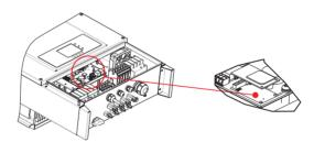
**Step 3** Screw out the sealing nut corresponding, to let the antenna expose a portion, and tighten the screw nut.
