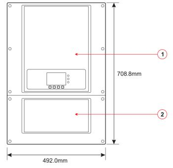
1 power converter part 2 wiring box
