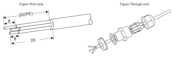
**Step 2** Insert sealing plug into housing, and tighten the screw nut.
