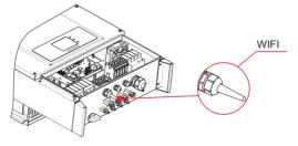
**Note:** Pull the WIFI antenna out a little bit to enhance the signal.
