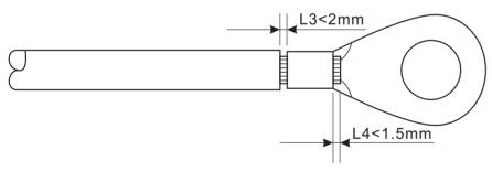
Note 1: L3 is the length between the insulation layer of the ground cable and the crimped part.L4 is the distance between the crimped part and core wires protruding from the crimped part.
