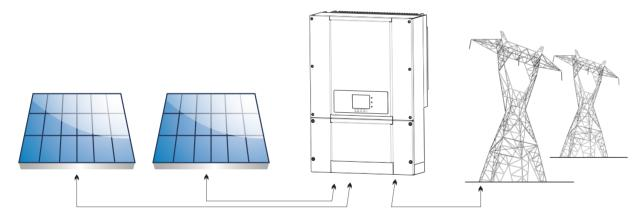
The inverter can be used only with photovoltaic modules that do not require one of the poles to be grounded.
