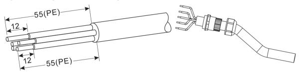
**Step 3** Connecting the AC output power cable: The AC output cable(R,S,T,N and PE) is connected to the terminal block, as shown in figure 4-7.
