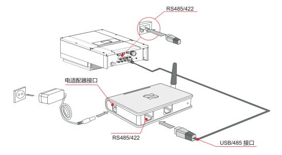
If multiple Sunny Horse Series are used, connect all Sunny Horse Series in daisy chain mode over the RS485 communication cable. First, set the RS485 address according to chapter 6.3 "Set address" part and SWT2(Match Resistance).
