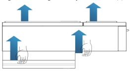
Step 2 Lift the Sunny Horse Series from the packing case and move it to the installation position.
