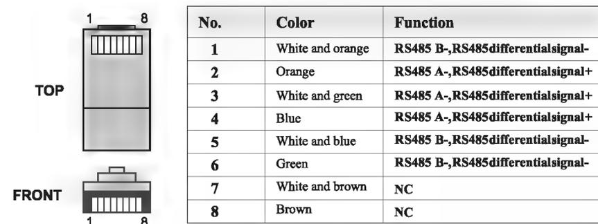
Figure 4-12 RS485 Connecting Communications Cables(2)
