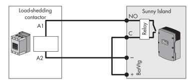
Figure 18: Connection of the control cable for one-level load shedding (example)
