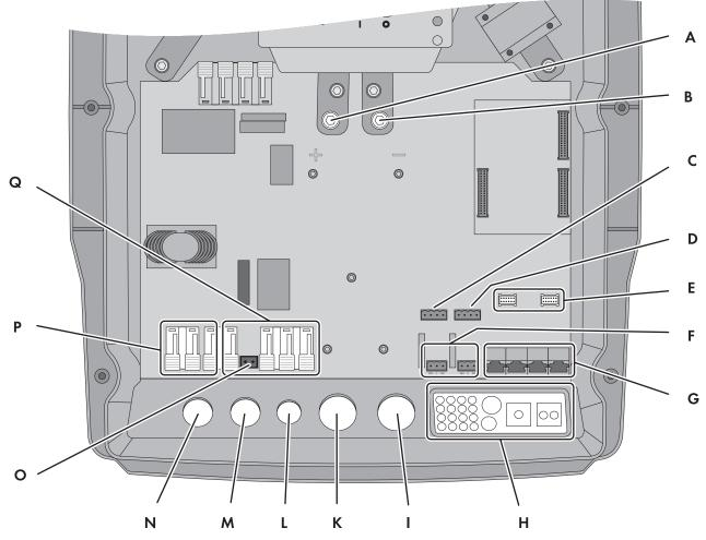
Figure 9: Connection area of the Sunny Island inverter
