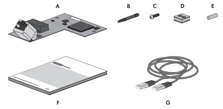
Figure 4: Components of the "Communication via Speedwire" order option
