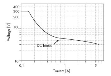
Figure 33: DC load limitation curve of multifunction relays 1 and 2
