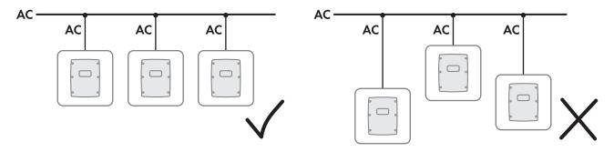
Figure 10: Correct, symmetric connection and incorrect, asymmetric connection of the Sunny Island inverters
