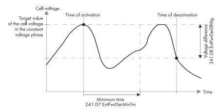
Figure 26: Switching-on time and switching-off time for utilization of excess energy during constant voltage phase
