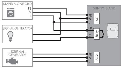
Figure 17: Connecting a signal generator to signal a generator request (example)
