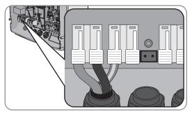
If the conductor cross-section of the grounding conductor is less than 10 mm<sup>2</sup>, make sure that an additional grounding conductor is connected to terminal AC2 Loads/SunnyBoys PE (see Section 7.5.3 "Connecting the Grounding Conductor", page 57).
