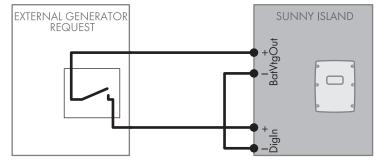
Figure 19: Connection of the control cable of an external generator request (example).
