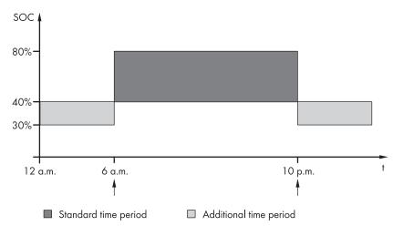
Figure 27: Profile of the SOC and the times for generator requests
