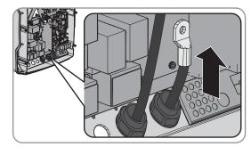
10. Route the **DC-** cable on the side of the protective cover marked with a - symbol.
