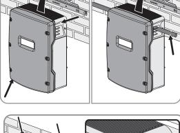
7. Use an Allen key (AF 5) to attach the Sunny Island to the wall mounting bracket on both sides with the M6x10 screws provided (torque: 4 Nm to 5.7 Nm). This will prevent the Sunny Island from being lifted off the bracket.
