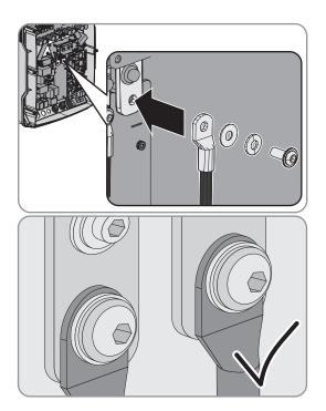
12. Tighten the swivel nuts of the cable glands (torque 4.5 Nm).
