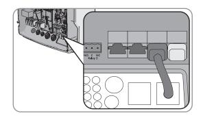
2. Ensure that the communication bus is closed at each end, e.g., with a terminator.
