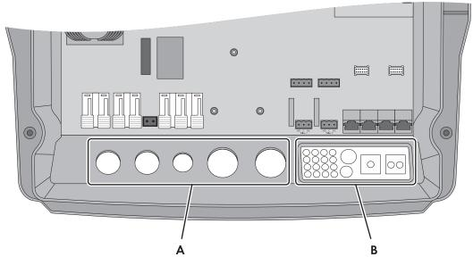
Figure 20: Position of the cable glands and the cable feed-through plate.
