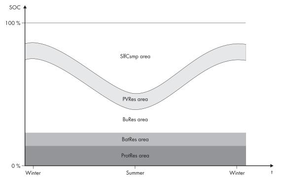
Figure 23: State of charge ranges of the battery according to the time of year (example)
