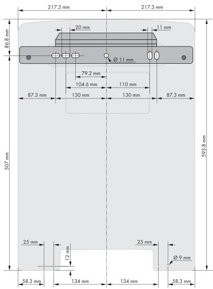
Figure 8: Dimensions of the wall mounting bracket and dimensions of the drill holes for the optional anti-theft device on the Sunny Island inverter enclosure
