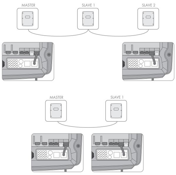
Figure 11: Internal communication cabling
