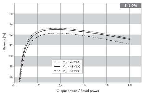
Figure 29: Characteristic efficiency curve
