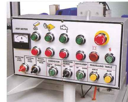
CENTRALIZED CONTROL PANEL
