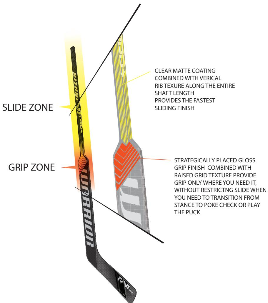
CLEAR MATTE COATING COMBINED WITH VERTICAL RIB TEXTURE ALONG THE ENTIRE SHAFT LENGTH PROVIDES THE FASTEST SLIDING FINISH
