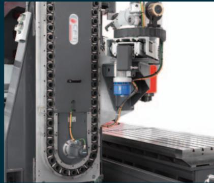
**Tool magazine:** available with turret configuration on 3-, 4- and 5-axis version, or with alongside column configuration on 4- and 5-axis version. Tool change on turret configuration with dual arm grippers at the X-axis limit, with 40 tool stations (optional 80). Tool change on the alongside configuration fast and safe, all along the X-axis and at the extreme limit of the Z- and Y-axis. Up to 120 tool stations. An external tool changer „tower“ is available upon request.
