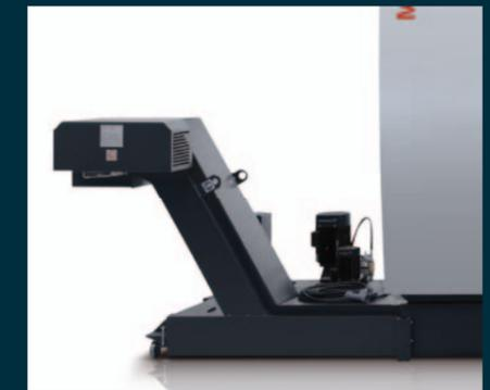
**Hinge type conveyor:** The chip rinsing system washes chips into the hinge type conveyor, which then automatically transports the chips from the machine into the customer provided container.
