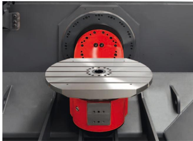
**Swivel-rotary table.** The swivel-rotary table has a large clamping area of 750 x 600 mm (29.5 x 23.6") and can bear loads of up to 300 kg (661.3 lb). This makes it possible to simply machine workpieces with an edge size of 530 x 530 x 417 mm (20.8 x 20.8 x 16.4"). The special shape of the table allows the spindles to move closer to the table center.
