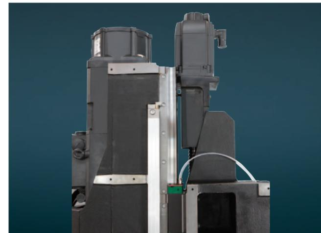
The direct drive on the Z-axis stands for highest accuracy and prevents any play of pulleys or belts.
