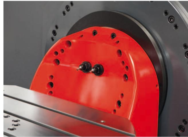
**Table rinsing system:** 2 nozzles for automatic rinsing of the table and workpiece from chips during processing in any table's position.
