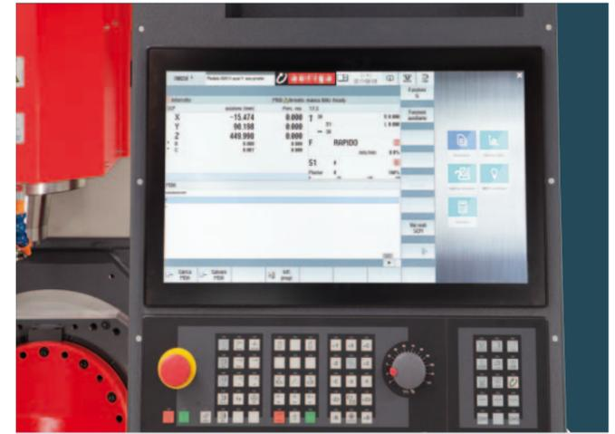
**The Sinumerik 840D sl incl. Shopmil.** The Sinumerik 840D sl incl. Shopmil is a universal and flexible CNC system and offers free contour programming, moving cycles for complex contours, fast reference point setting with touch probe systems, tilting the working plane, cylindrical surface machining, 3-D tool compensation, fast execution through short block processing times.
