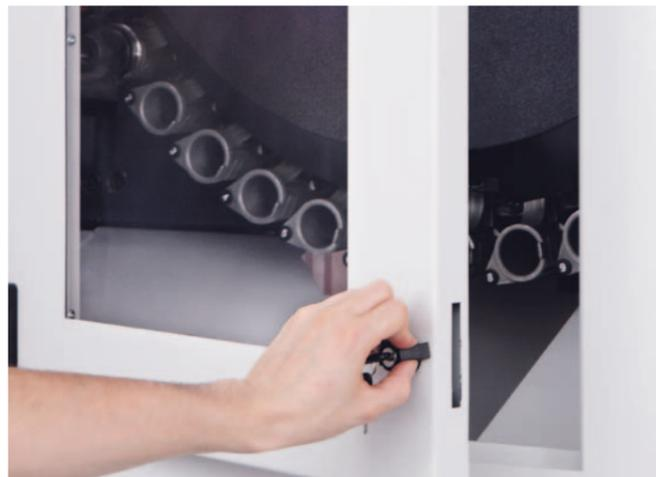
**Tool changer.** The tool changer is a drum magazine for 30 tools. A tool magazine with 40 or 60 tool stations is as option available. The tools are managed according to the variable tool stationcoding principle (random), which means that tools are always deposited in the first free magazine station for time reasons.
