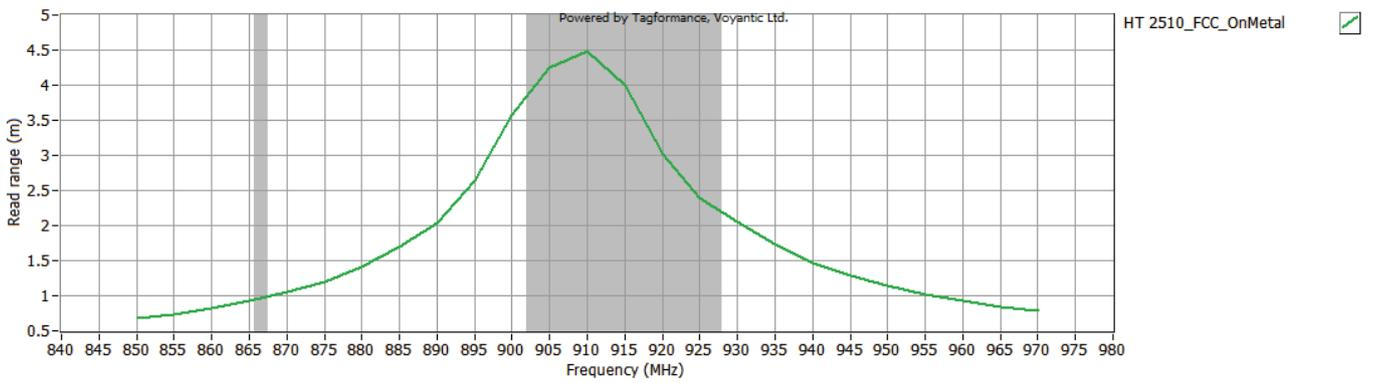
\*\* The indicated read range values are measured in our laboratory testing environment, where antennas with optimum directivity are used with maximum allowed operating power. Different surface materials and environments may exhibit different results.
