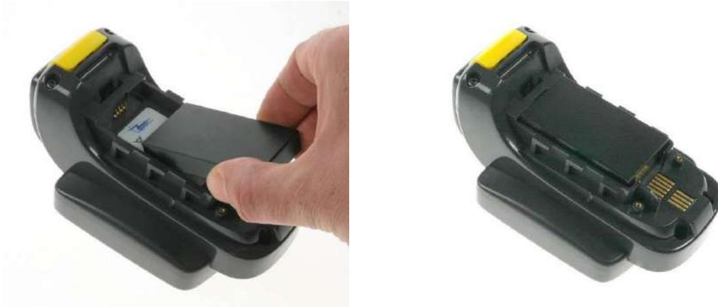
**FIGURE 6:** Battery Placement
