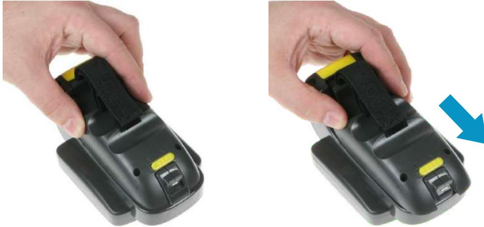
**FIGURE 4:** Slide Battery Cover
