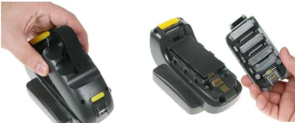
**FIGURE 5:** Remove Battery Cover
