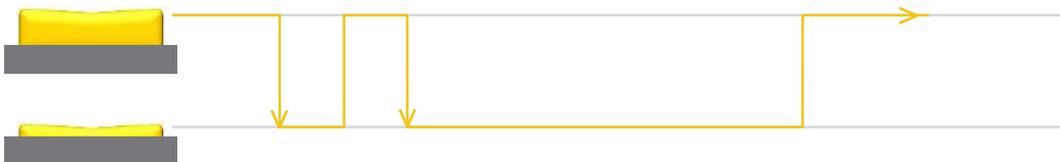
The secondary button click is a single click quickly followed by a second press (press-release-press).
