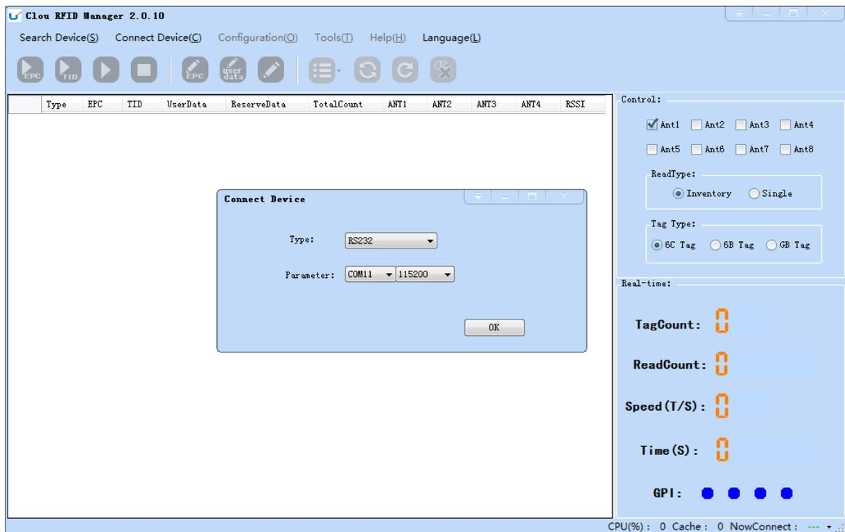
Image 4-6 Serial communication connection
