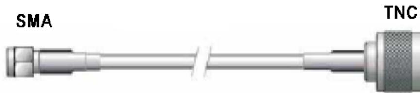
Picture 2-10 RF cable schematic chart
