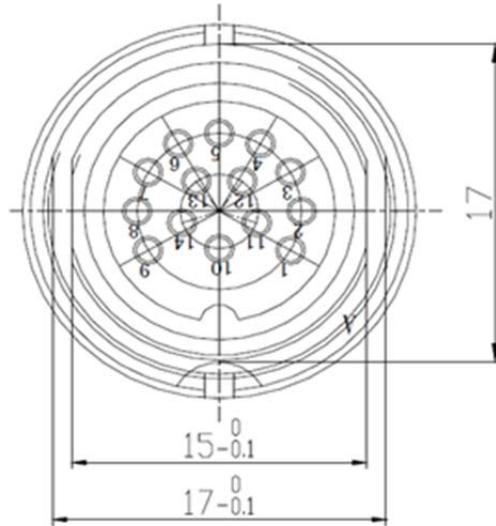
Picture2-7 Power supply & communication aviation plug chart
