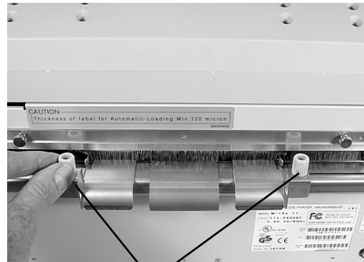
Label Width Adjustment Thumbscrews
