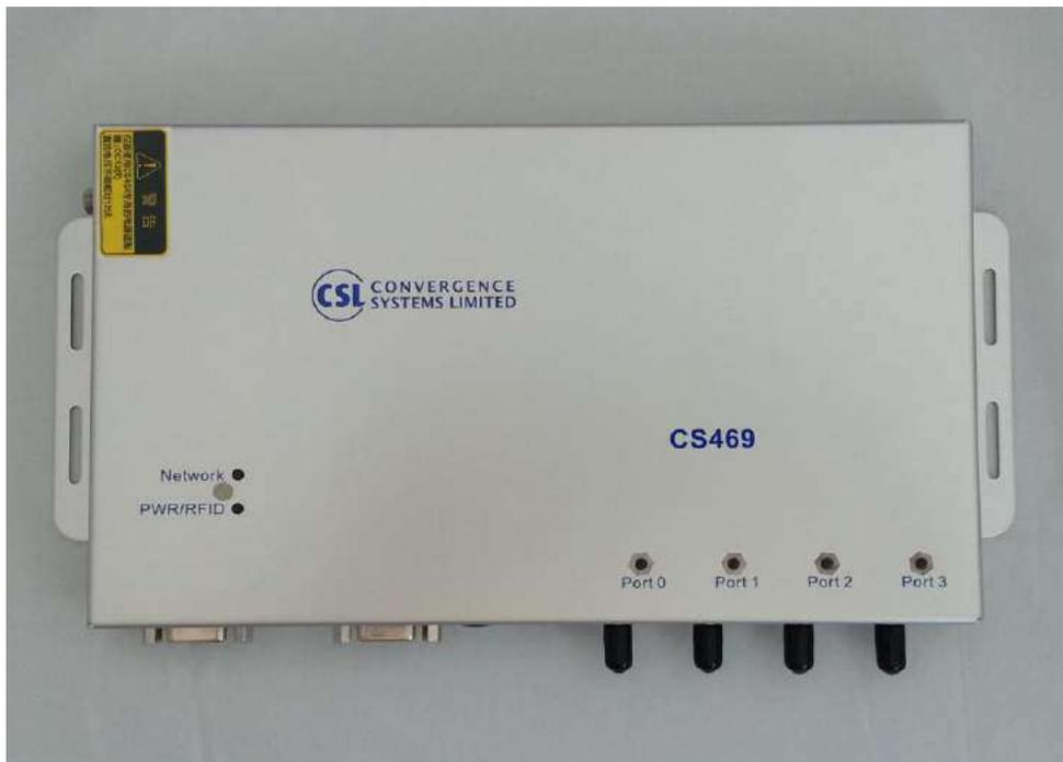
Figure 4-1 CS469 Reader Top View
