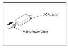
1. Plug the Mains Power Cable into the AC Adaptor
