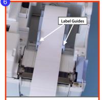
Install the label roll and position the sides of the labels under the Label Guides. Close the Top Cover and the printer is ready for use.
