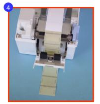
4. Thread the label backing paper underneath the black rollers and out of the front of the printer.
