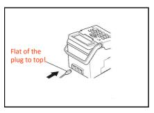
2. Plug the DC Output plug into it's socket at the rear of the printer.
