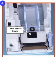
Clean the Label Sensor cover using a wipe.
