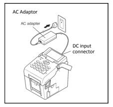
3. Plug the Mains Power Cable into the Mains supply socket.
