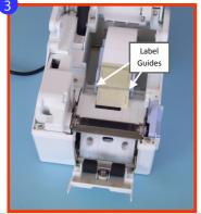
3. Fit the label roll into the printer and remove the first few labels from the backing paper. Position the edges of the roll underneath the two label guides.
