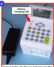
Connect the AC Power Adaptor to the printer and to the mains power supply The charge LED will illuminate to indicate charging and go out when the battery is fully charged.
