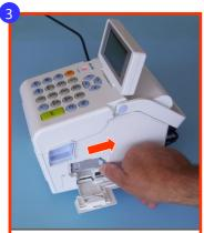
Lower the Battery Compartment Cover on the right-hand side of the printer.
