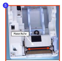
Clean the length of the rubber Platen Roller. Rotate the roller to clean the whole surface.
