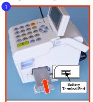
Put the terminal end of the battery into the compartment first. Push the battery inwards until it is locked in place by the Blue Locking Tab. Close the battery cover.
