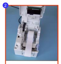
Ensure that the cover is in the "up" position. Remove the label roll.
