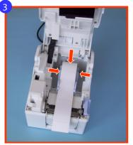
Place the new label roll into the Media Compartment. Labels upwards.
