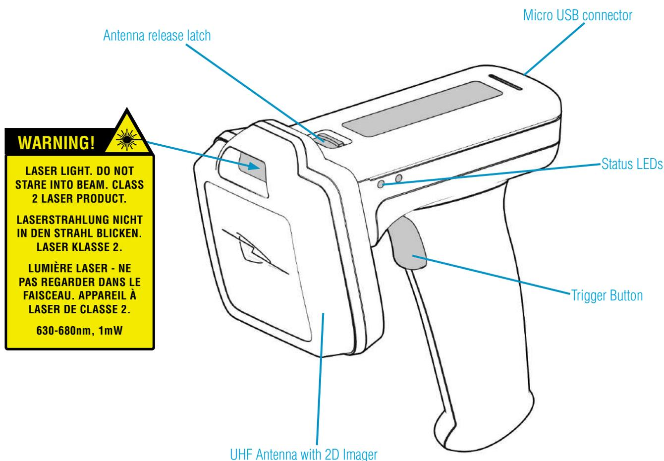
figure 1: Parts of the 1128 UHF Reader
