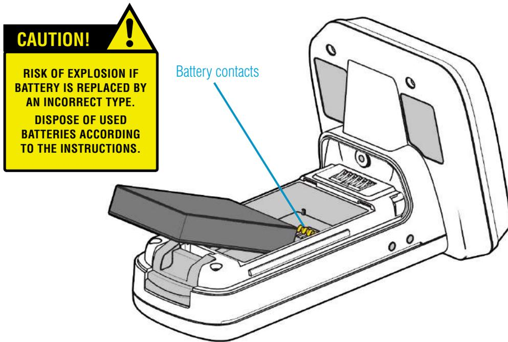
Figure 7: Battery placement
