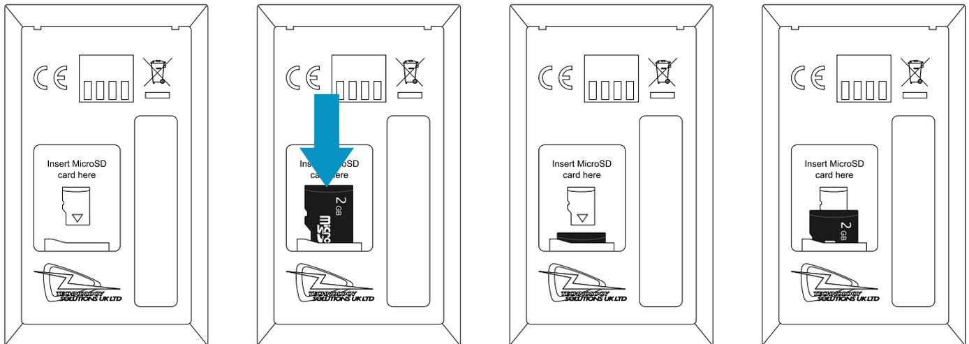
Figure 29: Micro SD Card Insertion and Removal
