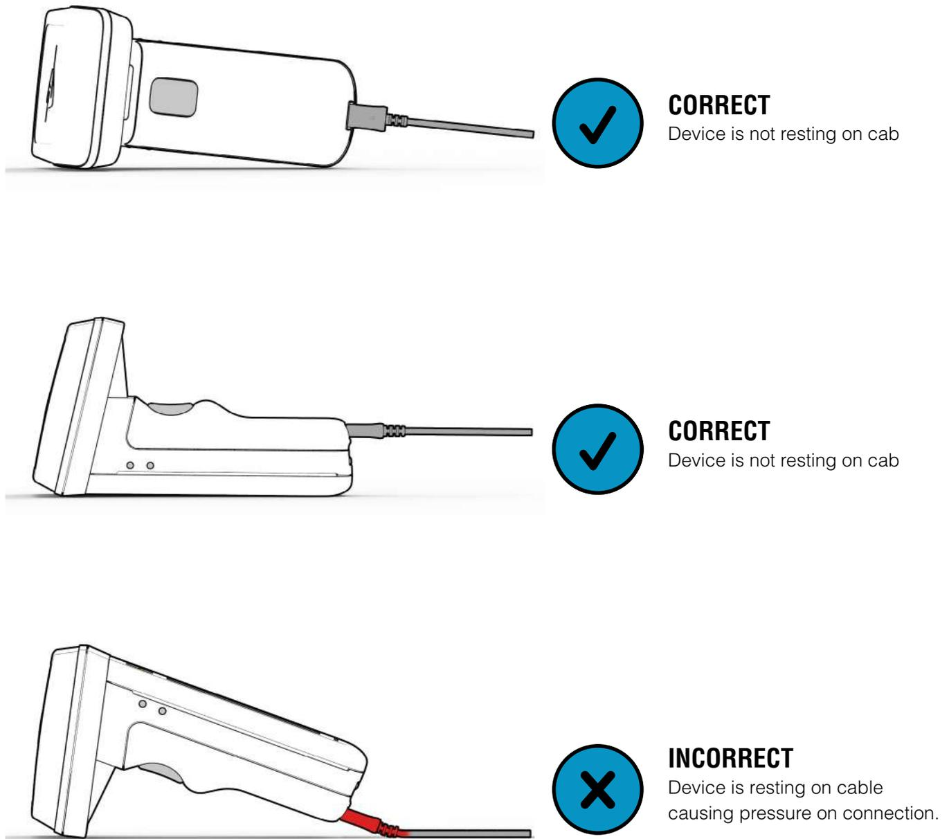
Figure 15: Micro USB cable and UHF reader orientations
