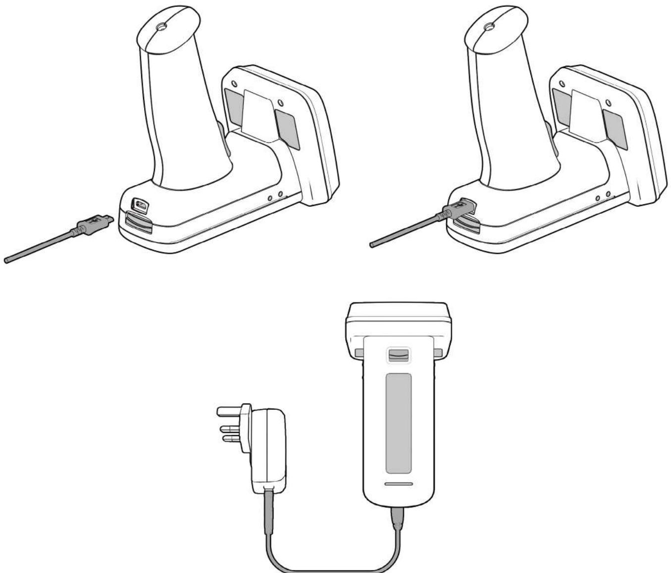
Figure 14: Attaching the Micro USB cable
