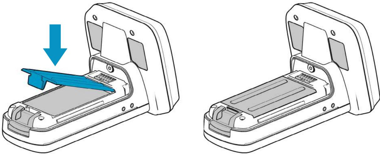
Figure 9: Replace battery cover
