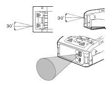
IrDA communication is limited to a 15 to 20 cm range. The usable range may vary depending on the usage environment, or the capabilities of other IrDA devices. Communication is compromised by direct sunlight or ambient light. In such a case, block the strong light from entering the IrDA filter, or reduce the distance between the two IrDA ports.
