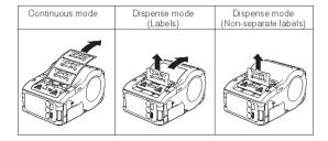
You can select **Dispense mode** for non-separate labels by using the printer setting tool.
