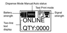
**Battery strength:** Three-segment indicator. When all segments are lit, voltage level is greater than 8.0 V. Two segments indicator a level of between 7.8 V and 7.9 V. One segment indicates a level of between 7.6 V and 7.7 V. When all segments are off (voltage level below 7.5 V, printing is not possible.)
