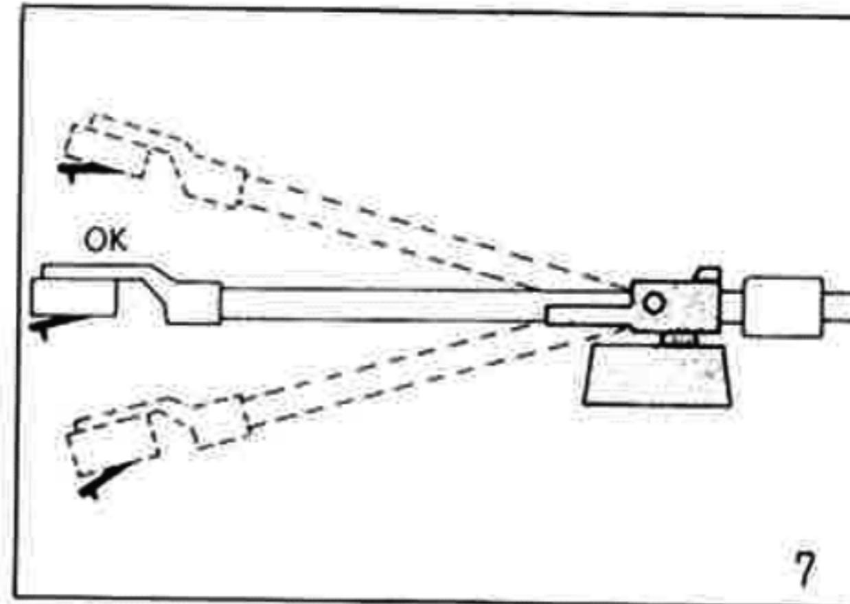
Lift the tonearm off the tonearm rest and place it to the left of the arm rest (viewed from the front). Turn the counterweight until the tonearm balances horizontally (fig. 7). Return the tonearm to the arm rest and clamp it with lock-lever of the rest.
