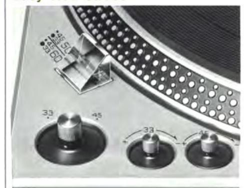
Two sets of strobe markings appear on the tapered rim for 33-1/3 and 45 RPM, at both 50 and 60 Hz synchronization, with either type of AC source. The prism strobe lamp lights when power is turned on, thus serving as a pilot lamp. The combination of prism lamp and tapered strobe rim results in easy viewing from any position.
