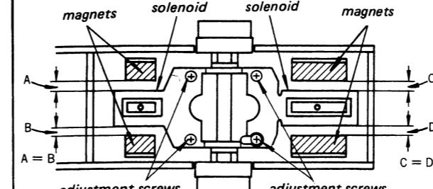
3. After the adjustment, tighten the adjustment screws.
