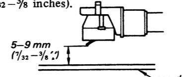
3. If necessary, loosen the adjustment screw (M3 x 3) and adjust the arm lifter height.
