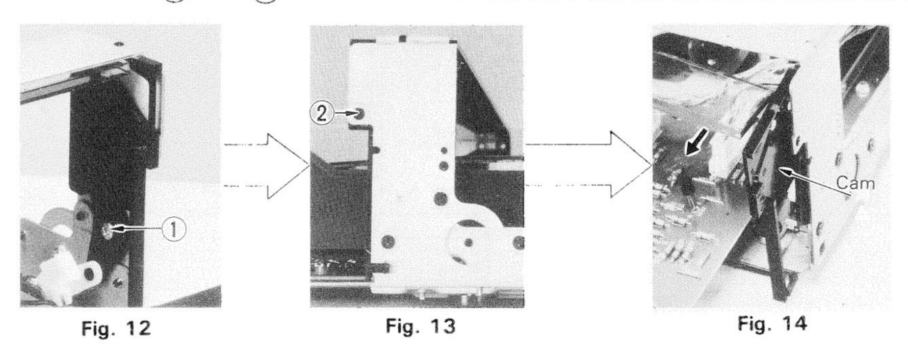
2. To attach the door, reverse the procedure. Push the door lever by hand and insert the projection (A) into the slot.
