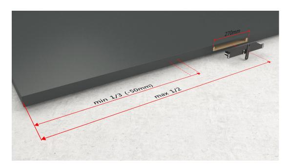
From a technical point of view, we advise to position the pivot axis between 1/3 (-50mm) up to the center of the door leaf width.
