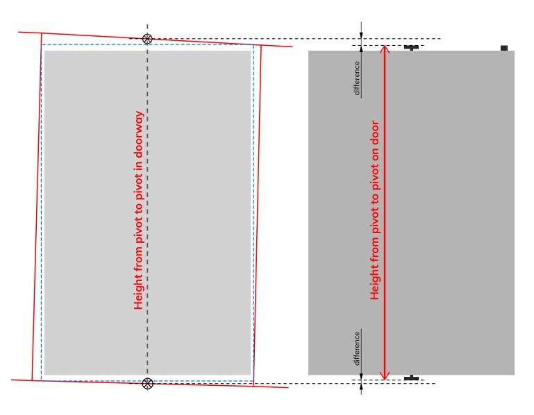
Check the pivot height of the door with the doorway measurements, and synchronize them if necessary.
