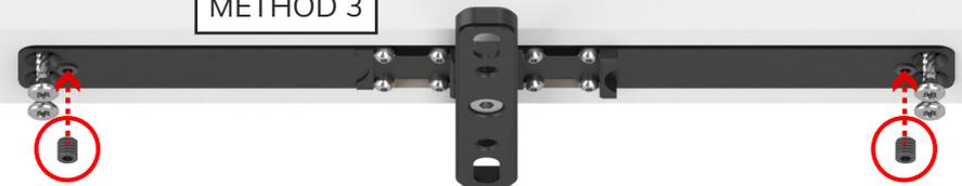
3. Adjust the inbus screws to move the hinge further away from the door leaf (loosen 4 hinge screws first). (only possible for non compressable door structure)
