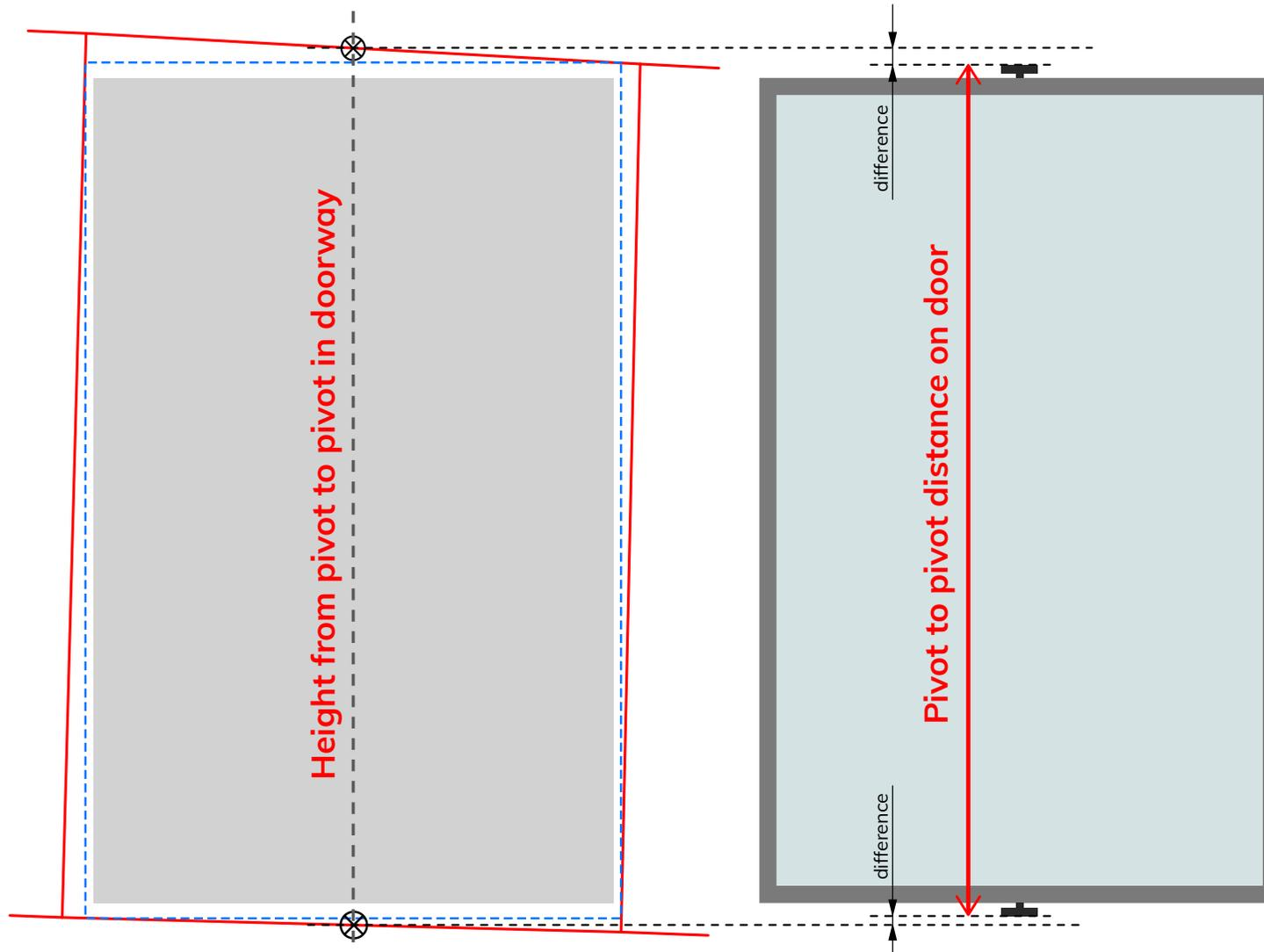
Compare the pivot to pivot distance of the door with the measured doorway height at the axis point.
