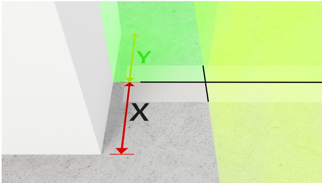
Position the second laser plane exactly on the desired door leaf center location.
