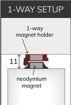
If 1-way operation is needed, use the 1-way accessory instead (also with the magnet inside).
