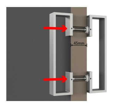
Insert the handle with its 2 rods into the door leaf, and place the other handle on the other side over the rod ends.
