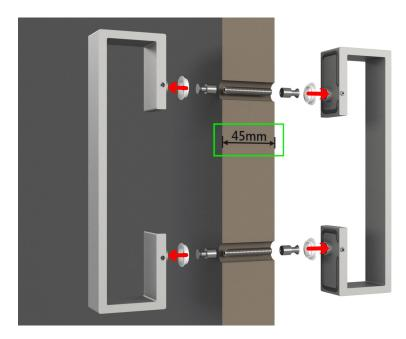
Slide the nylon bushings over the door handles as shown.
