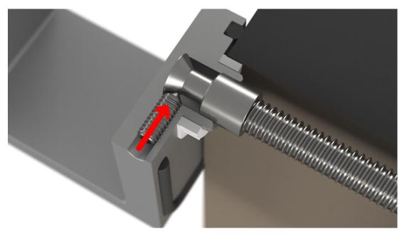
Tightening the 2 inbus screws will pull both handles closer to each other, locking them firmly to the door leaf.
