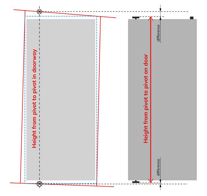
Check the pivot height of the door with the doorway measurements, and synchronize them if necessary.
