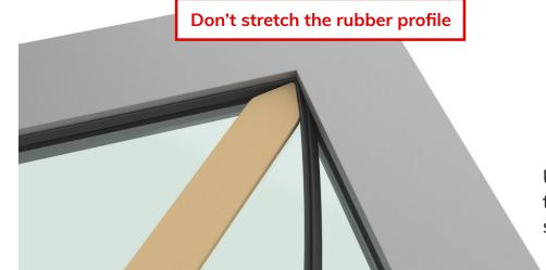
Use a wooden tool to press the rubber tightly (90°) into the corners without stretching it.
