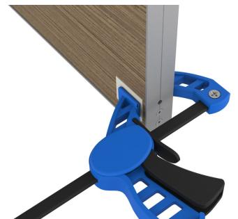
Firmly press both sides together, for example using a quick grip tool.
