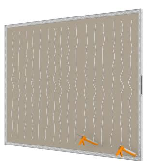
Apply Fix All on the 5045 frame and filling material.
