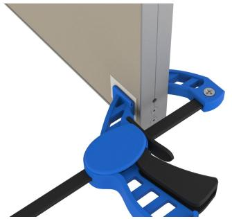
Firmly press both sides together, for example using a quick grip tool.
