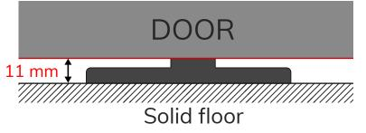
2. Use supplied shims between floor and hinge (= less stable).
