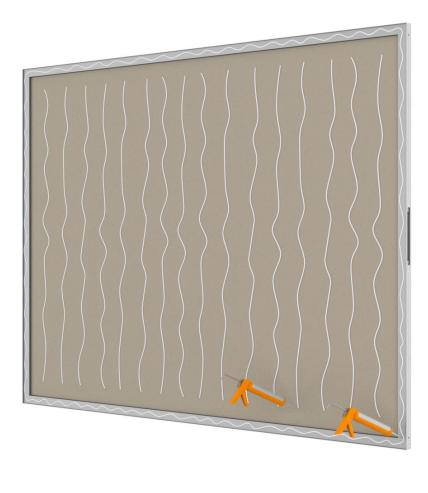
Apply Fix All on the 5045 frame and panel.
