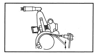
Adjust the throttle cable adjuster until there is specified free play on the throttle cable.
