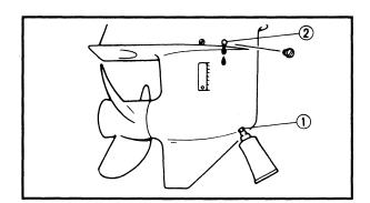
• Fill the gear oil through the drain hole until it overflows at the level hole.
