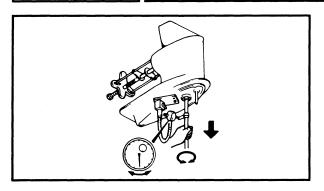
Attach the dial gauge on the lower case, and make the dial gauge stem contact the mark on the indicator.
