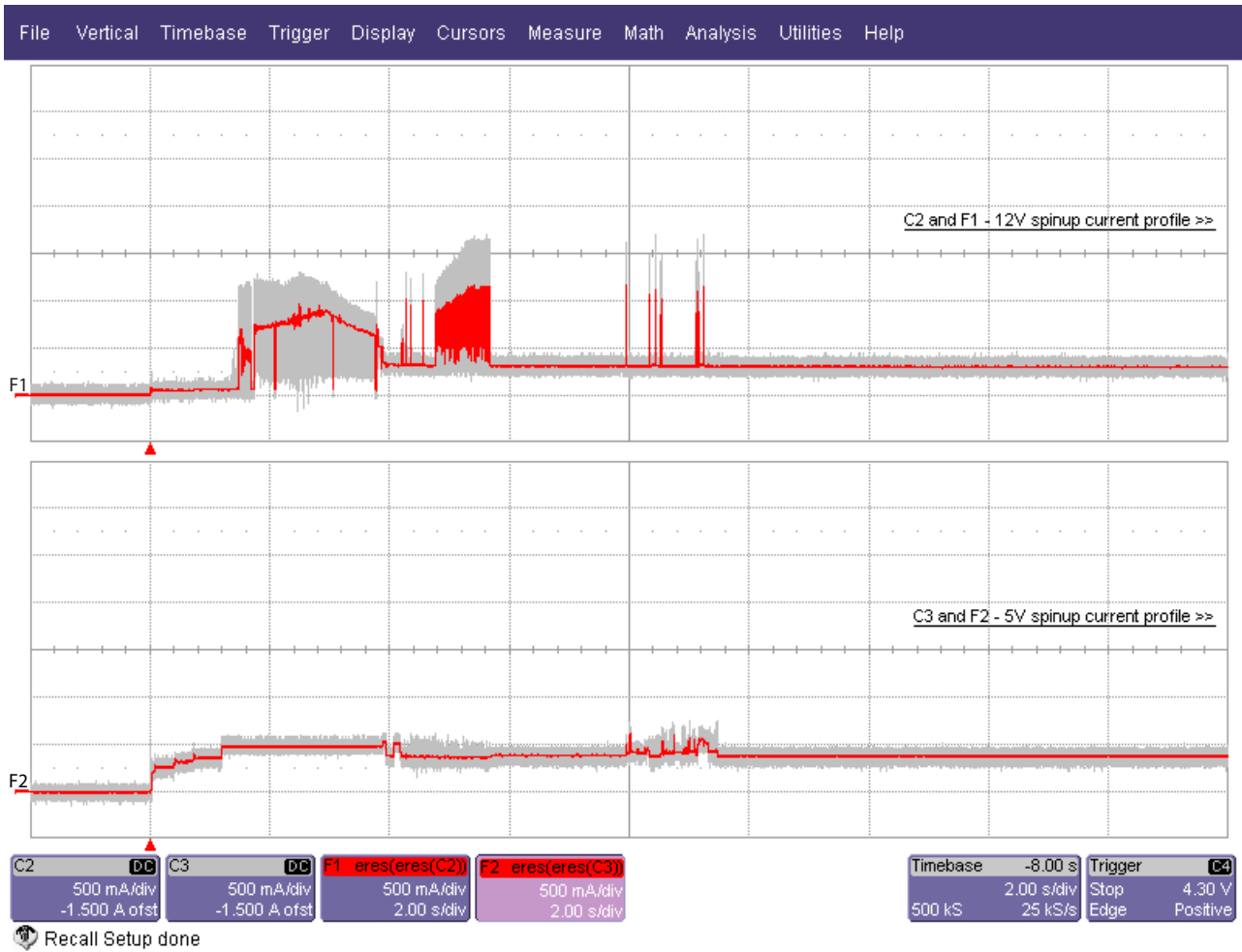
Figure 16. Current profiles for 600GB models
