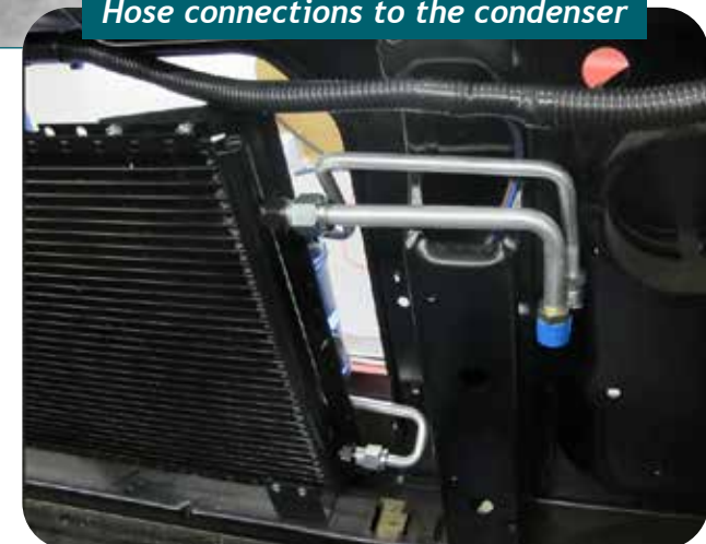
Hose connections to the condenser
