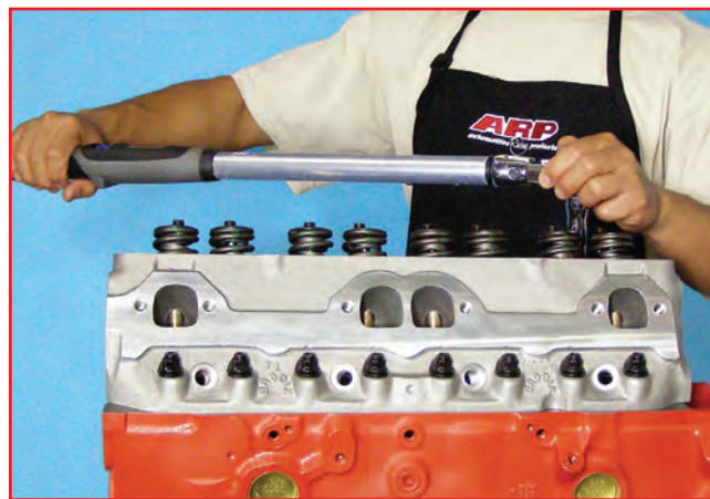
5. Following the engine manufacturer's torque sequence, tighten the bolts to the recommended torque value found on the instructions provided with each kit.
