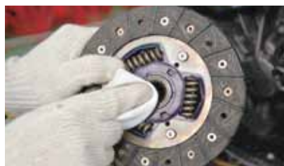
⑤ Remove Excess Grease
