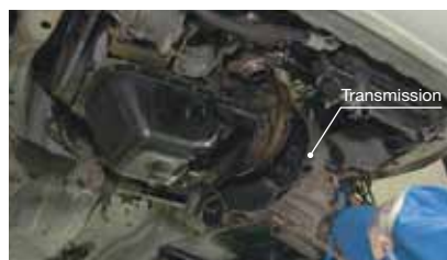
⑩ Reinstalling the Transmission
