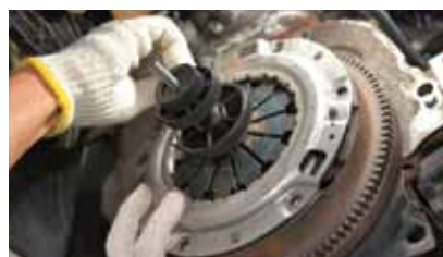
⑦ Installing to Fly Wheel
