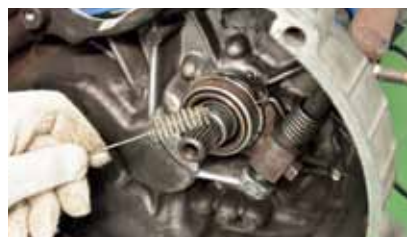
④ Apply the Grease to Top Shaft
